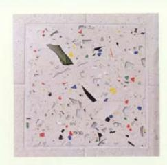
Right: A tall slot window in the children's bathroom provides privacy while letting in light. The bathroom surfaces are Syndecrete, a concrete solid-surfacing material developed by Hertz. Syndecrete is a mix of cement and recycled materials, including fly ash (a waste product from coal-burning electric utilities), glass, reground plastic, and scrap metal. Hertz also used Syndecrete for the kitchen counters, fireplace, and much of the furniture in the house.
